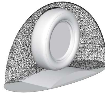
Part of the acoustic FE mesh
